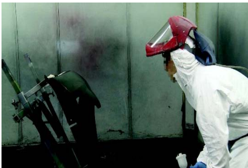
Lifted Visor to Inspect Product from HSE RR1064
