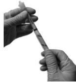
3. Holding the ampoule in an upright position, with the fill tip pointed upwards, squeeze the ampoule towards the top of the tube to break the internal glass ampoule. A cracking sound is heard when doing this. **DO NOT BEND THE TUBE.** (See Diagrams 2 & 3).
